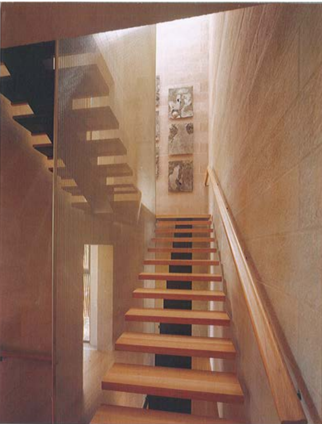
ABOVE: Speck suspended a stainless-steel mesh curtain in the main stairwell, balancing the solidity of the limestone walls. The material, he explains, "has a buttery feel—not harsh or cold, very warm. We cut and sandblasted it to give it a soft, irregular texture." The bronze panels are by Darcy Miro.
